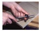
2. Using a rat-tail file, file any roughness or ridges off the inside of the hoop. This step is very important.
