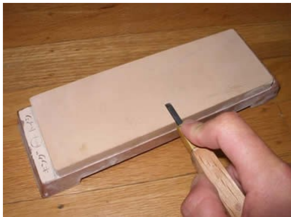
First, start by sharpening the backside of the chisel. This is the flat, un-beveled side.
